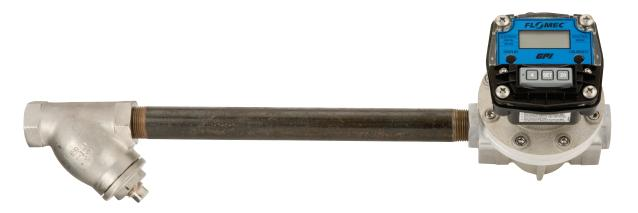
Oval Gear Meters work best with clean fluid, free of debris. GPImeters carries Y Strainers to fit most models of Oval Gear Meters. These strainers range from 1/4 in. to 2 in. models. All sizes come complete with blow-off and plug.
